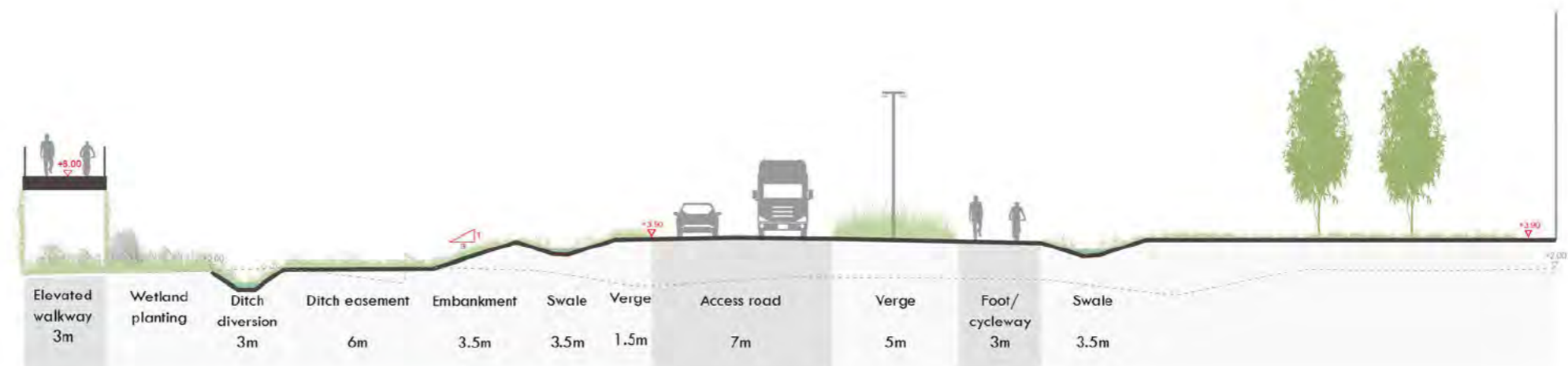
Figure 5.13: Illustrative section through main access road
