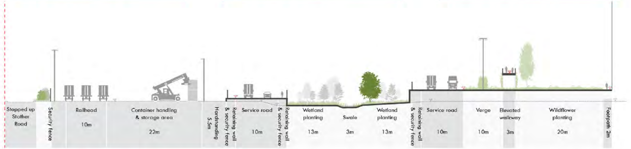
Figure 5.21: Illustrative Railhead and Rail Corridor Sections
