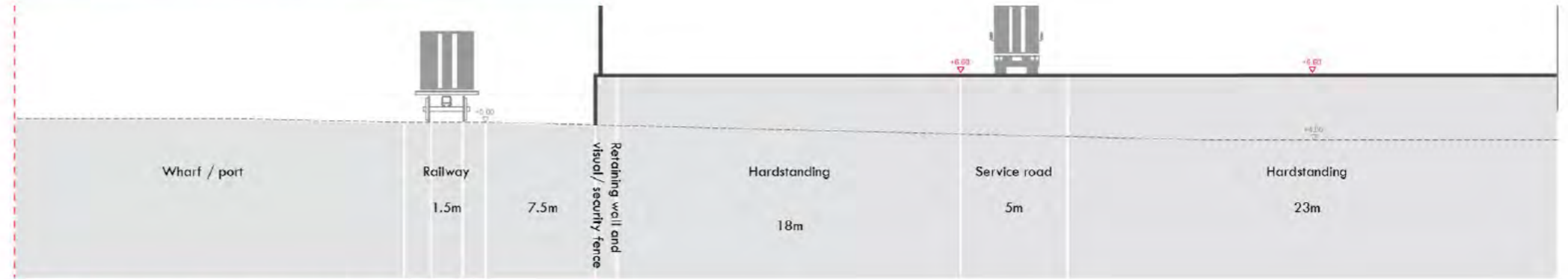
Figure 5.22: Illustrative Railhead and Rail Corridor Section
